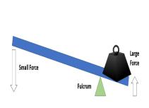
Can be used to make a small force lift a heavier load. A lever always rests on a pivot.
