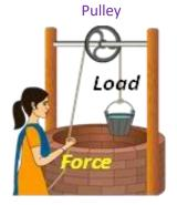
Can be used to make a small force lift a heavier load. The more wheels in a pulley, the less force is needed to lift a weight.
