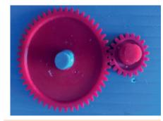
Gears or cogs can be used to change the speed, force or direction of a motion. They turn in opposite directions when connected.
